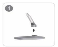
Insert the Stand Connector into the Stand in the direction shown by the figure.
